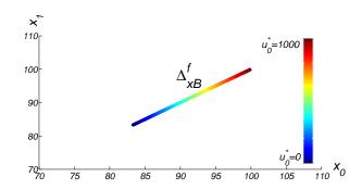
Fig. 5. Numerical example for the set  $\Delta_{xB}^f$  (color line). The left end of the line corresponds to the input flow vector:  $u_0^*=0$ ,  $u_1^*=0$  while the right one is for  $u_0^*=1000$ ,  $u_1^*=0$ .
