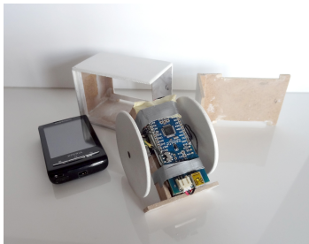
Figure 6: Assembly of the components of Stackables in a wooden box.
