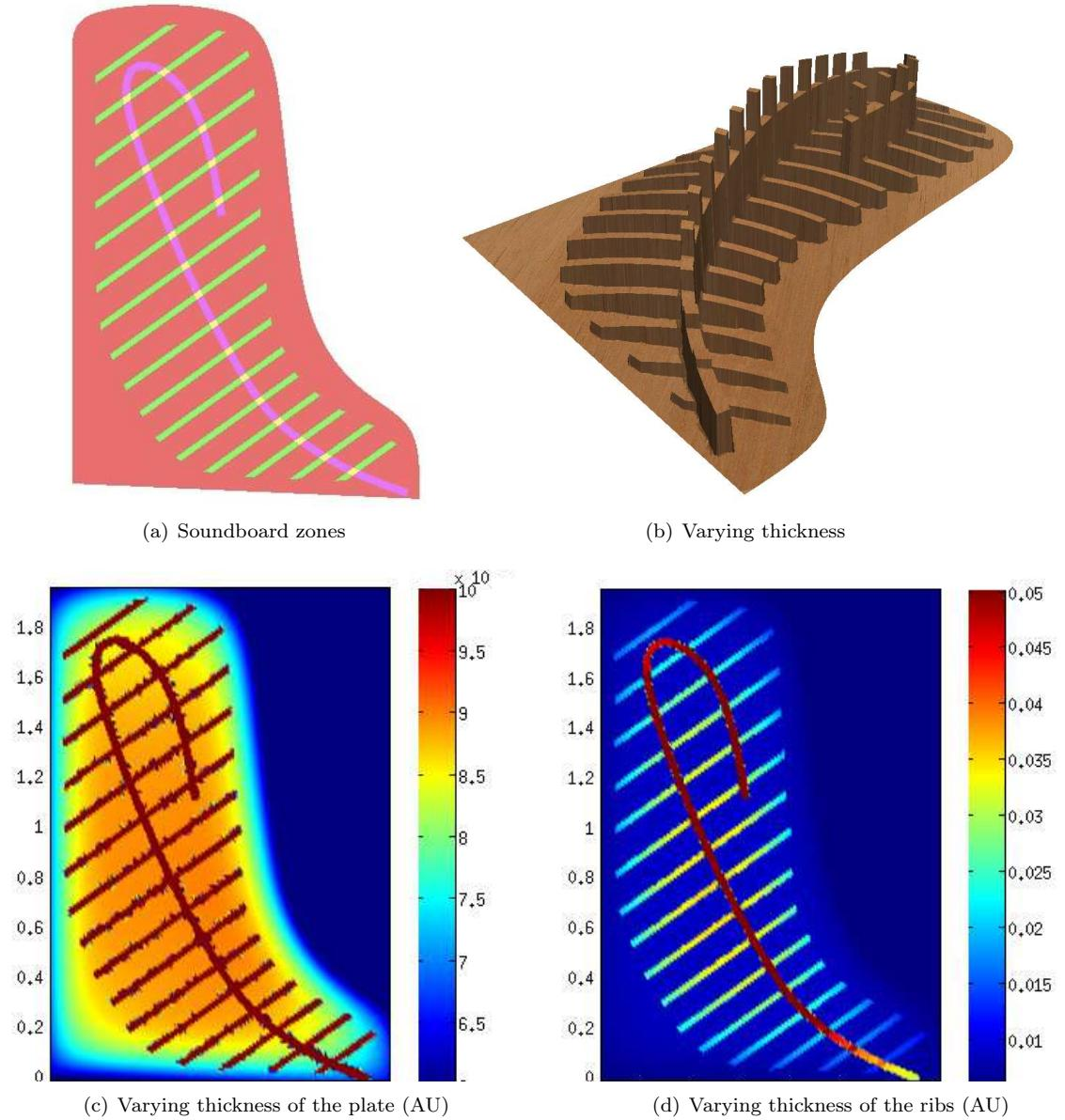
Figure 2: Different soundboard zones : different materials, orthotropic direction, and thicknesses.
