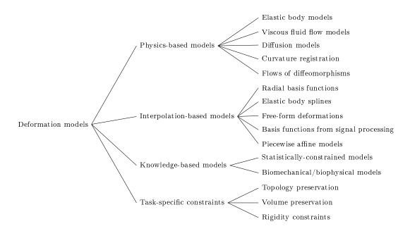
Figure 1: Classification of deformation models.
