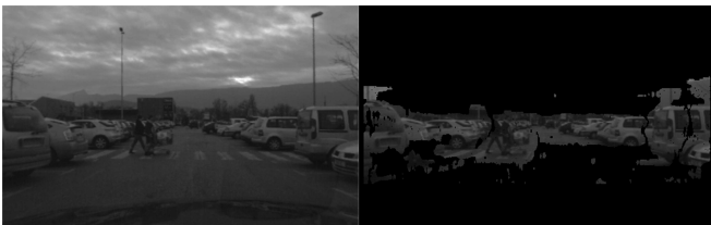
Fig. 2. Depth mask example. The mask filters out the road surface and the objects that are over a prespecified height.
