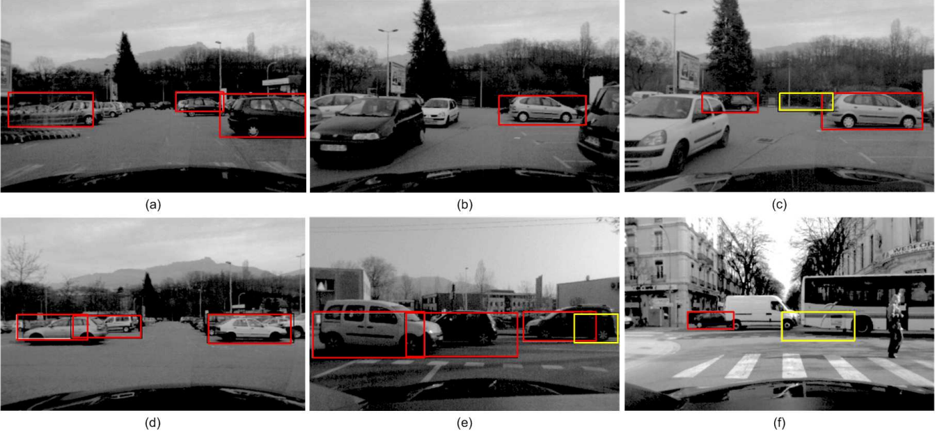
Fig. 6. Car-side detection examples. True and false positive detections are represented with red and yellow bounding boxes respectively. (a) Cars in different scales with significant background clutter and significant occlusions are detected. (b) Precise detection of the un-occluded vehicle, whereas a vehicle that is heavily occluded in the left is not detected. (c) Difficult detection of a vehicle which is far and partially occluded and a false detection in the region between the road surface and the trees. (d) Detection with partial occlusion. (e) Partial detection of a taller than normal vehicle (on the left). The training dataset does not contain vehicles of this type. (f) Successful detection of a partially occluded car and a false positive arising from a bus and a van. Training separate detectors for these type of vehicles as well will help to avoid these false alarms.
