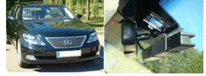
Fig. 5. Our Experimental Platform. Lexus LS600h vehicle equipped with a TYZX stereo camera placed behind the windshield.
