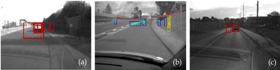
Fig. 10. Common sources of errors in detection using a laser scanner. (a): laser scanning plane intersects road surface. (b): non planar road is seen as an obstacle. (c): laser temporal tracking failed. All of these errors are correctly discarded by the stereovision-based validation step.
