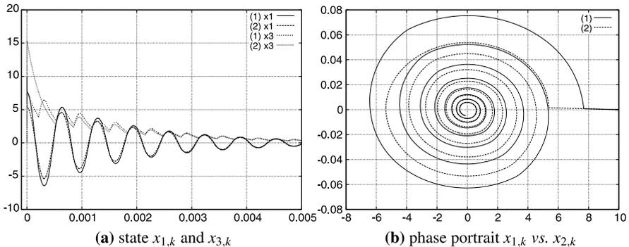
**Fig. 14.8** Simulation of the configuration in Fig 14.5 with (1) the scheme (14.43) and (2) the scheme (14.25)  $\theta = 1/2$ ,  $\gamma = 1/2$
