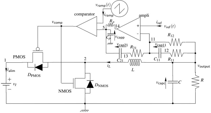
Fig. 14.9 Buck converter
