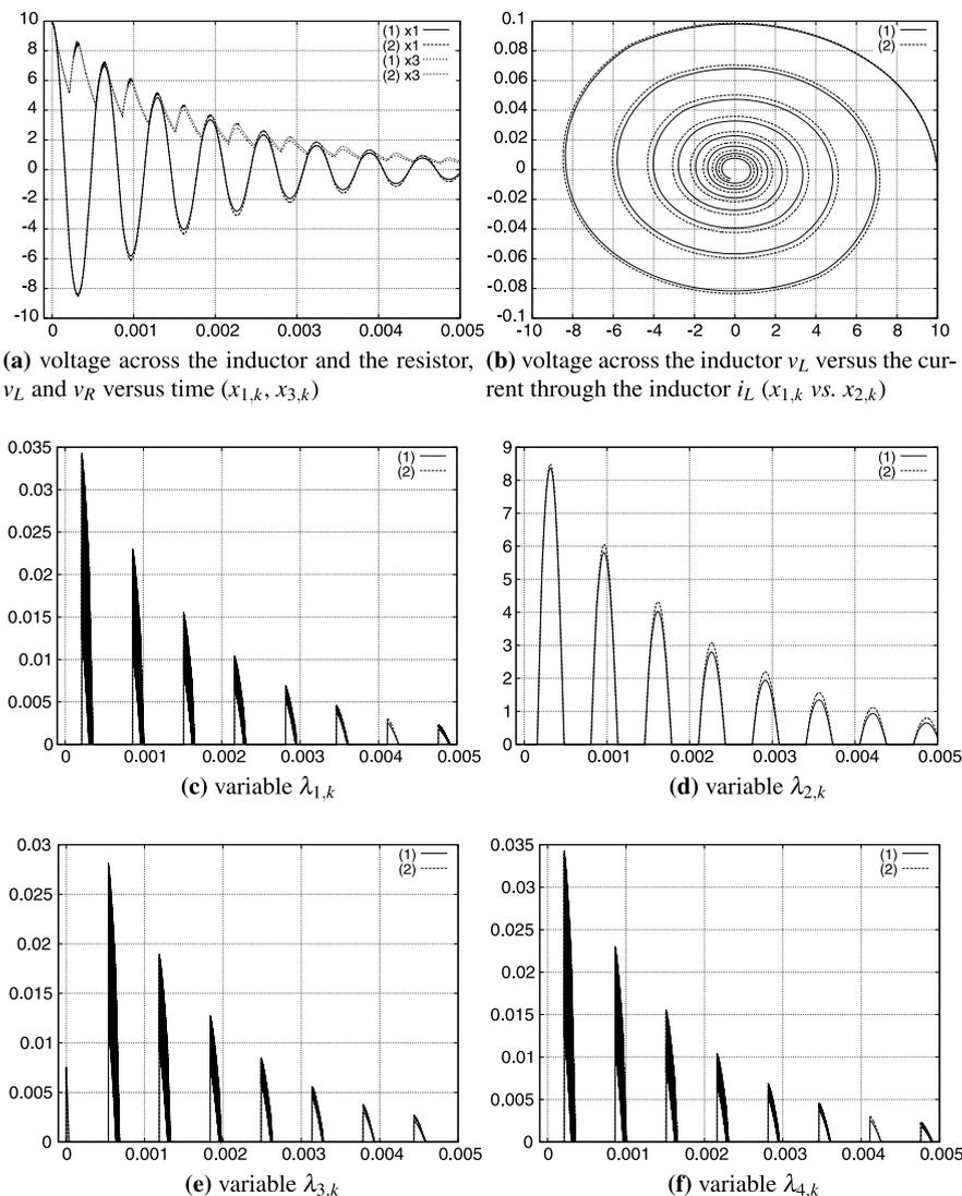
**Fig. 14.7** Simulation of the configuration in Fig. 14.5 with the scheme (14.25) for two values of parameters: (1)  $\theta = 1, \gamma = 1$ ; (2)  $\theta = 1/2, \gamma = 1/2$ . Some instabilities are generated for the approximation of the BV functions
