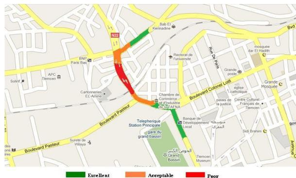
Figure 1. Signal quality associated to a cognitive radio
