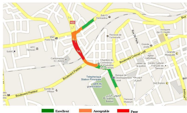
Figure 1. Signal quality associated to a cognitive radio
