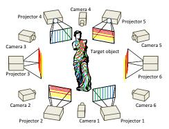
Figure 1. A setup example to reconstruct the entire shape using six projectors and six cameras.
