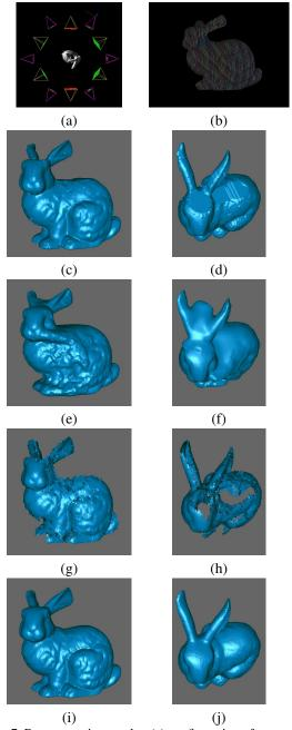
Figure 7. Reconstruction results: (a) configuration of cameras and projectors, (b) synthesized image, (c)-(d) recovered shape with our technique, (e)(f) recovered shape with MVS [2], (g)(h) recovered shape by Furukawa *et al.* [4], and (i)(j) ground truth.
