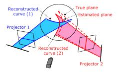
Figure 4. Projector-camera-projector(PCP) case
