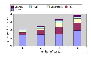
**Fig. 3.** Cycles Per Instruction breakdown of  $\mu$ server, by number of cores.
