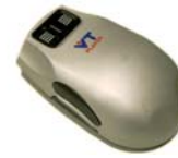
Figure 1. The VTPlayer tactile mouse
