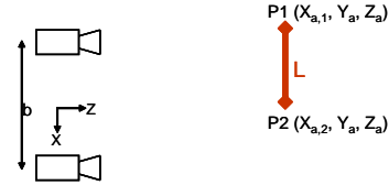
Fig. 6. Observed object, parallel to the images planes.
