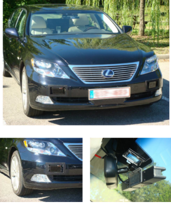
Fig. 7. Experimental vehicle with the lidar sensors (bottom-left) and the stereo-vision camera (bottom-right).
