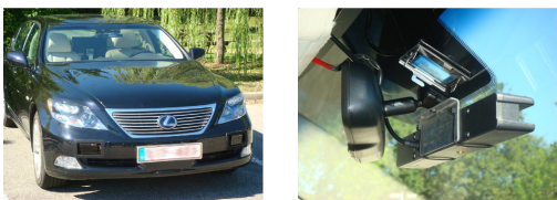
Fig. 5. The experimental vehicle is a Lexus LS600h, equipped with a TYZX stereo camera, and two IBEO Lux laser scanners.
