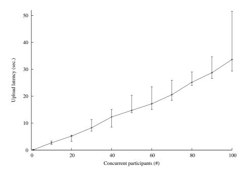
Figure 7: Impact of concurrent uploads on ANTDROID.
