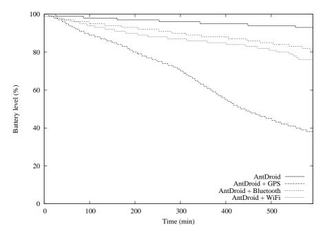
Figure 6: Impact of ANTDROID on the battery lifespan.
