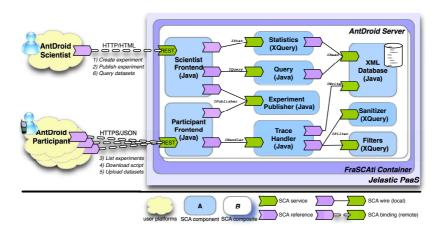
Figure 1: Architecture of the ANTDROID Software Platform.
