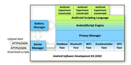
Figure 2: Architecture of the ANTDROID Software Architecture
