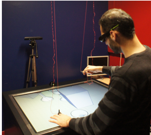
Figure 1: 3D object modeling by interacting on and above a multi-touch stereoscopic surface.
