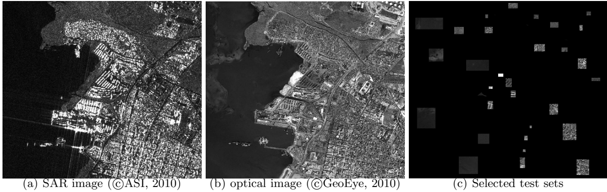
Figure 6. Original SAR image of Port-au-Prince in Haiti, coregistered panchromatic optical image and the selected ground truth used to test the results.
