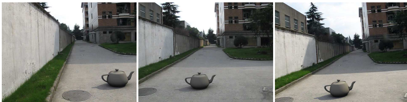
Fig. 1. Resulting integration of a virtual teapot into the building video sequence with moving viewpoints. The virtual teapot is lighted using a illumination model composed of sunlight and skylight. Thanks to our online tracking of lighting variations, the illumination is consistent from frame to frame between the real scene and the teapot.
