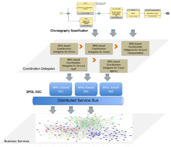
Figure 5-3. BPEL-based mapping of choreographies.
