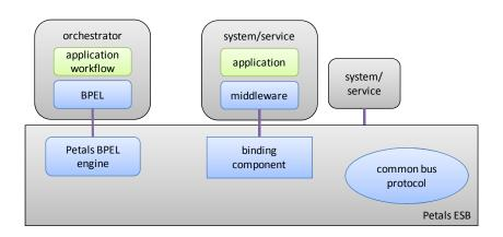
Figure 4-6. Workflow-based system orchestration on the PEtALS ESB.
