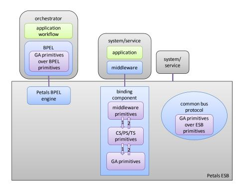
Figure 4-7. Extended orchestration supporting heterogeneous interaction paradigms.
