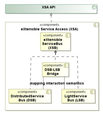
Figure 4-1. Service access mechanisms of the CHOReOS middleware.
