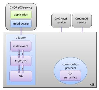
Figure 4-4. XSB support for multiple interaction protocols/paradigms.
