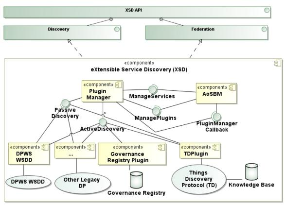
Figure 3-1. Service discovery mechanisms for the CHOReOS middleware.
