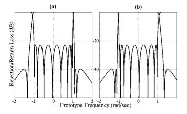
Fig. 8. (a) Original and (b) inverted rejection and return loss performance of an 8-3 asymmetric characteristic in extended box configuration.
