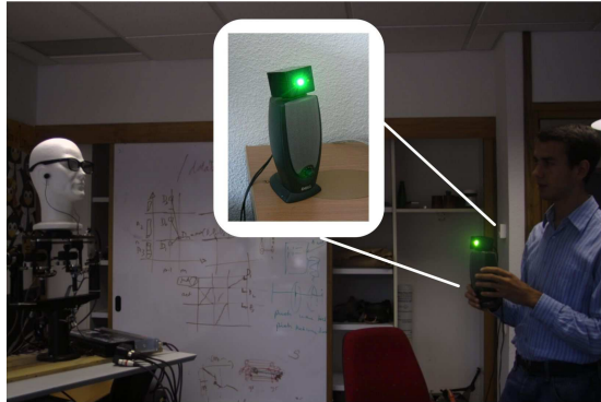
Figure 3: Audio-visual device used to align the auditory and visual spaces. An LED light bulb is mounted onto a speaker which makes the visual localization more precise. White noise is played throughout the recording to improve the auditory localization.
