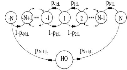
Fig. 1. One dimensional cell, rate partitioning and user's movement
