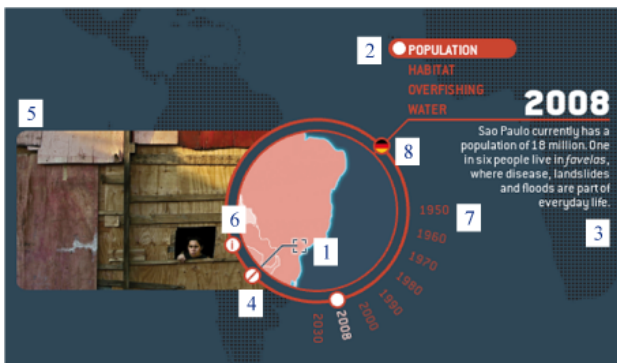
Figure 3. Screenshot of GeoLens showing the user interface components: (1) Geolocated point of interest; (2) Map view menu; (3) Geolocated text; (4) Open/close button for geolocated images and videos; (5) Geolocated image; (6) Open/close button for map legend; (7) Time slider for population data; (8) Language toggle.
