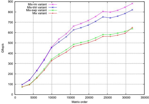
Figure 5. Algorithmic optimizations for static SGETRF on **Tesla-C1060**
