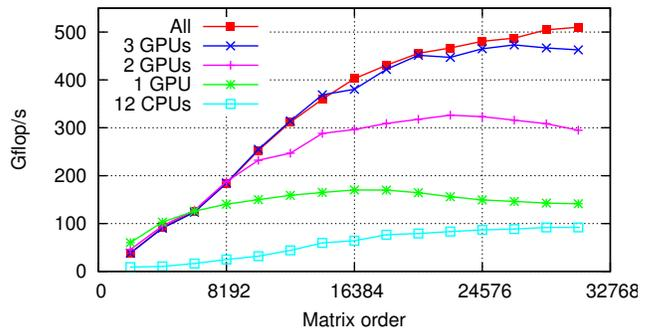
Figure 9. Scalability of dynamic DGETRF on **Fermi-C2050**
