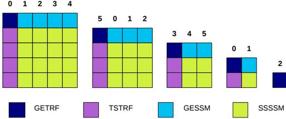
Figure 2. Task partitioning across six processing units.
