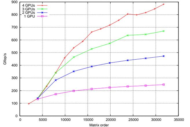
Figure 6. Scalability of static SGETRF on **Tesla-C1060**
