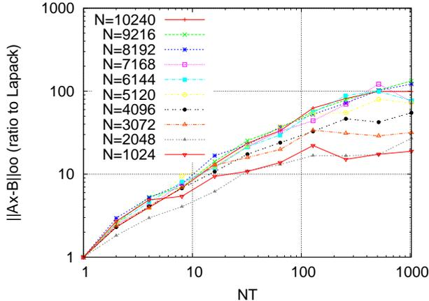
Figure 8. Numerical accuracy of the residual ( $\|Ax - b\|_\infty$ , logarithmic y-axis) when the number of tiles per row ( $t$ , logarithmic x-axis) varies, for random matrices  $A$  of various orders  $N$  in double precision. The residual is normalized to the residual obtained with LAPACK.
