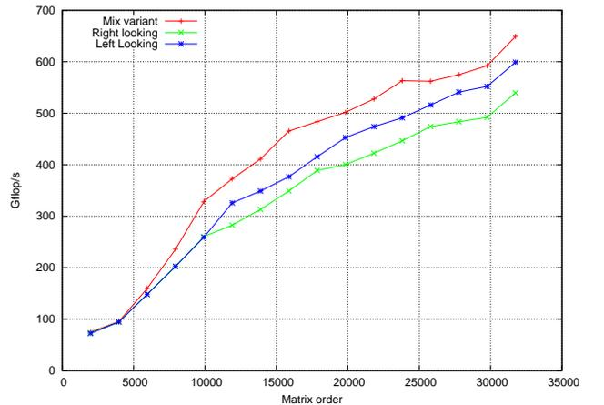
Figure 4. Looking variants for static SGETRF on **Tesla-C1060**
