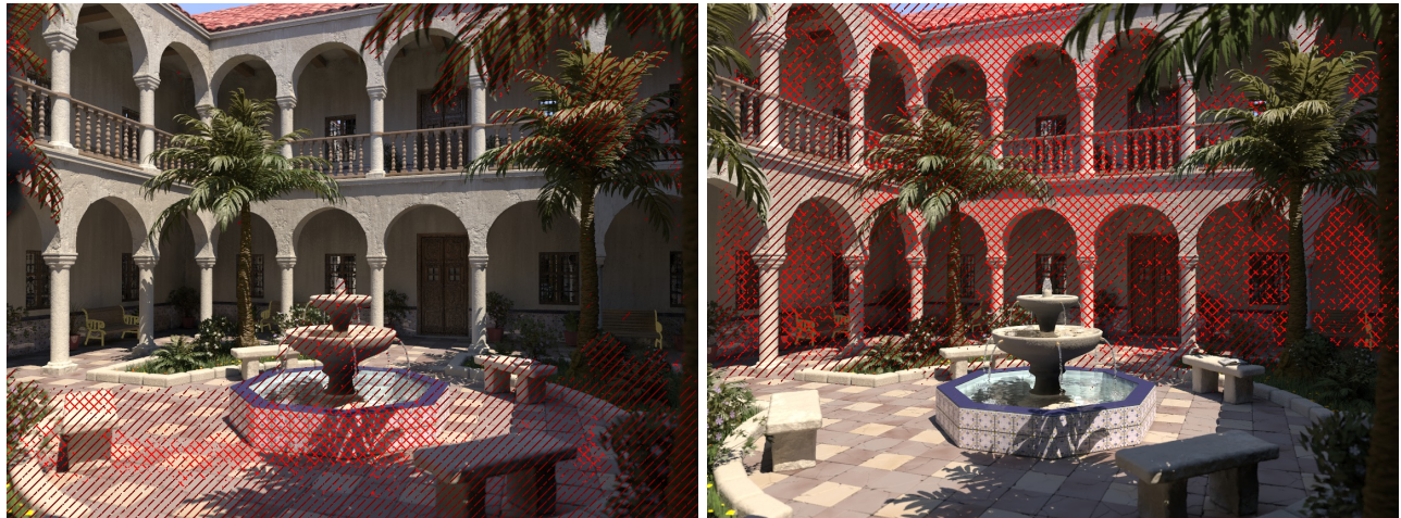
Figure 12. The original images from the (LFar, RNear) test case with zebra stripes on the regions of the image which are less focused than in the other image: Left red zebra area (e.g. the fountain) is less focused than in the right image. Right red zebra area (e.g. the background) is less focused than in the left image.
