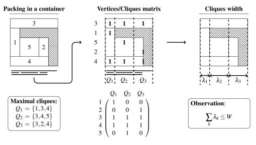
Fig. 4: A strip decomposition w.r.t. the first dimension of a 2d-orthogonal packing
