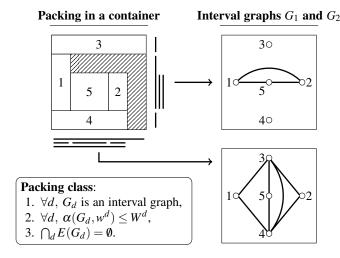
Fig. 2: A Fekete & Schepers' packing class with respect to a 2d-packing
