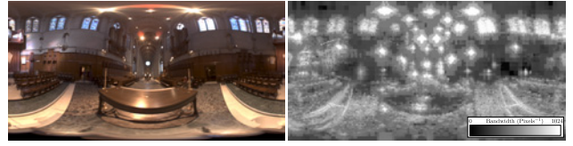
Figure 7: Input environment map and its local angular bandwidth computed using a 2D wavelet decomposition.
