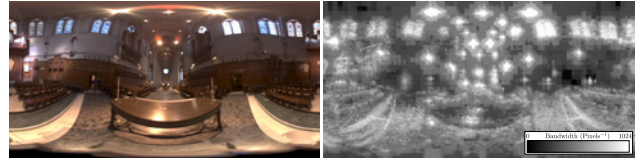
Figure 7: Input environment map and its local angular bandwidth computed using a 2D wavelet decomposition.
