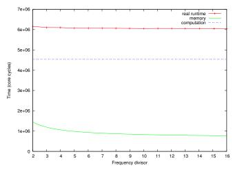
(a) Matrix-matrix product model: the cycle count is given according to the the core frequency divisor
