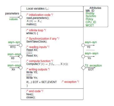
Figure 3: Algorithmic module structure.
