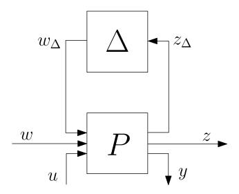
Figure 10: System under LFT form
