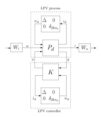
Figure 11: LFR control structure
