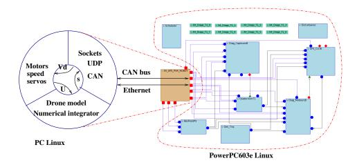
Figure 5: Hardware-in-the-loop structure.
