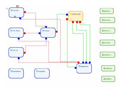
Figure 8: Decoupled LQ drone controller
