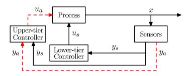
Figure 15: Two-tier control strategy (solid lines denote dedicated point-to-point, wired communication links and continuous sensing and actuation; dashed lines denote networked (wired or wireless) communication or asynchronous sampling and actuation).
