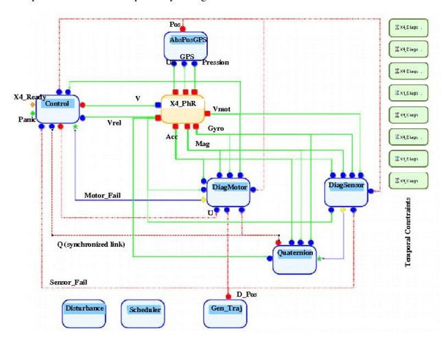
Figure 2: X4 drone control and diagnosis block-diagram.
