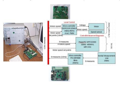
Figure 4: The quadrotor h/w bench-test.
