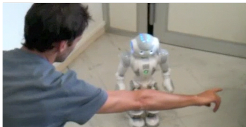
Figure 6: In this mode of interaction, the robot is guided by the hand and arm gestures made by the user. In order to have a robust recognition, we used a WOZ framework, where the wizard was only seeing through the robot’s viewpoint.
