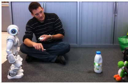
Figure 5: Users can drive the robot with a Wiimote. They can also draw its attention toward an object by pointing it with a laser pointer.
