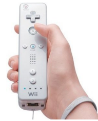
Figure 4: Users can move the robot by using the directional cross or directly orient the Wiimote to aim its head. However, the lack of feedback make it very difficult to estimate whether the robot really sees the object the user wants to teach it.
