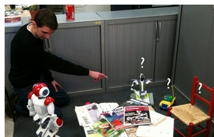
Figure 2: To allow users to designate a particular object to a robot in a cluttered environment, we need to provide them with a robust and accurate pointing detection. Otherwise it may lead to a restrictive interaction and even to false learning examples.
