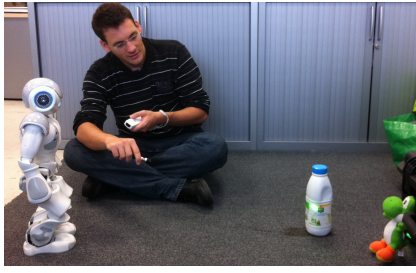
Figure 5: Users can drive the robot with a Wiimote. They can also draw its attention toward an object by pointing it with a laser pointer.
