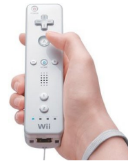
Figure 4: Users can move the robot by using the directional cross or directly orient the Wiimote to aim its head. However, the lack of feedback make it very difficult to estimate whether the robot really sees the object the user wants to teach it.
