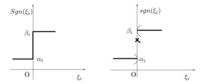
Figure 2: (a) The general relay characteristics. (b) The general relay single-valued map.
