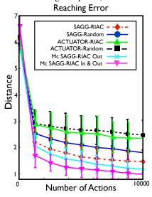
Fig. 5. Reaching errors estimated using different databases collected with different exploration methods on a over 10 quadruped experiments of 10000 actions
