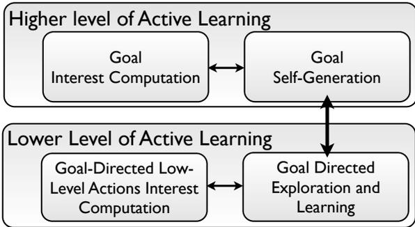
Fig. 1. Global Architecture of the SAGG-RIAC algorithm.
