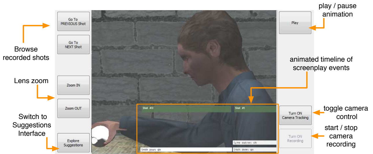
Figure 6: Screenshot of the interface in Camera Control / Movie Playing mode. The overlay horizontal bars show an animated timeline of screenplay events and their duration, together with an indication of the camera angle and framing that is currently being used in the movie.
