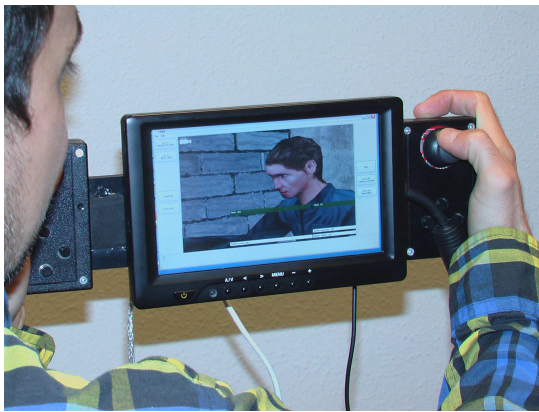
Figure 4: Our hand-held virtual camera device with custom-built dual handgrip rig and button controls, a 7-inch LCD touch-screen.
