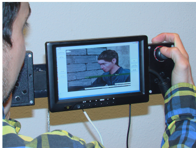
Figure 1: Our hand-held virtual camera device with custom-built dual handgrip rig and button controls, a 7-inch LCD touch-screen.
