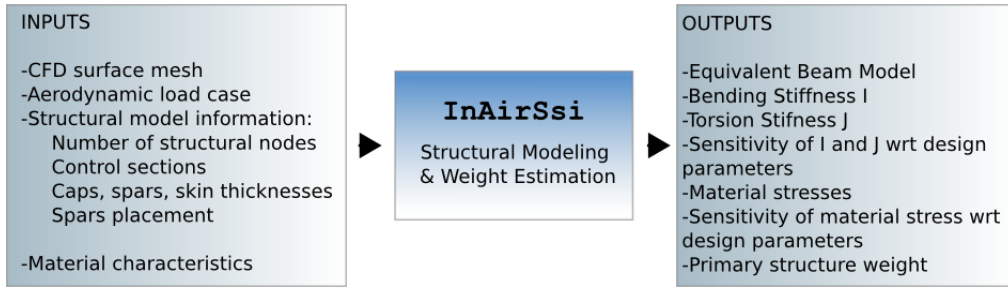
FIGURE 13: Input-output system of structural modelling tool
