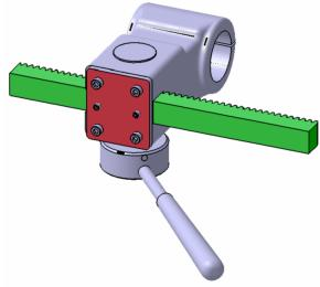
Figure 8 Drill support model.
