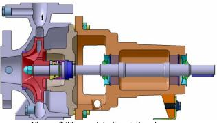
Figure 2 The model of centrifugal pump.
