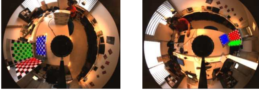
Figure 7: Images used in the SfM experiment with reprojected points superimposed (hyper-catadioptric).
