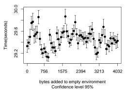
Fig. 2. Mean 95% Confidence Interval of some SPEC CPU 2006 Applications (compiled with gcc)
