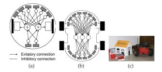
Fig. 5 (a) Braitenberg vehicle. (b) Conceptual Pioneer P2-AT. (c) Pioneer P2-AT robot with camera.
