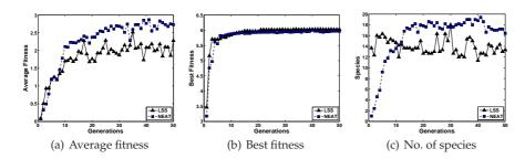
**Fig. 13** Performance plots that compare behavior-based speciation with the LSS measure and the NEAT method for the homing navigation problem with the Khepera robot. All plots are averages over the total number of runs.
