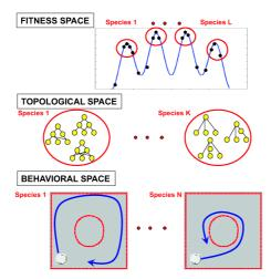
**Fig. 1** Speciation in neuroevolution can take place in different spaces for ER. The top row shows the basic niching technique carried out in fitness space, common in MOEAs. Next, speciation based on topological similarities between ANNs. Finally, the bottom row shows the proposed behavior-based speciation where each species has distinct behavioral traits.
