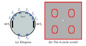
Fig. 4 (a) The Khepera robot, with eight proximity sensors and two motor actuators. (b) The 4-circle world, used as the second training environment for the navigation problem.
