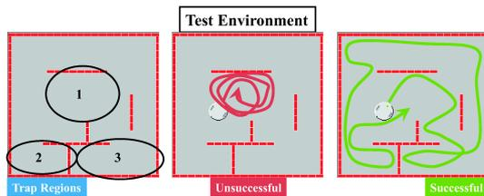
**Fig. 9** The *Test Environment*, from left to right: 1) The regions within the test environment where a robot controller can get **trapped**; 2) a sample behavior getting trapped in *region 1*; and 3) a behavior that successfully navigates without getting trapped.
