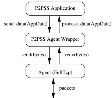
Figure 1: Simulator architecture.
