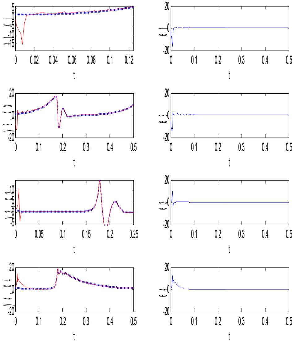
Figure 6: Synchronization of 4D chaotic system with impulsive control method for case II
