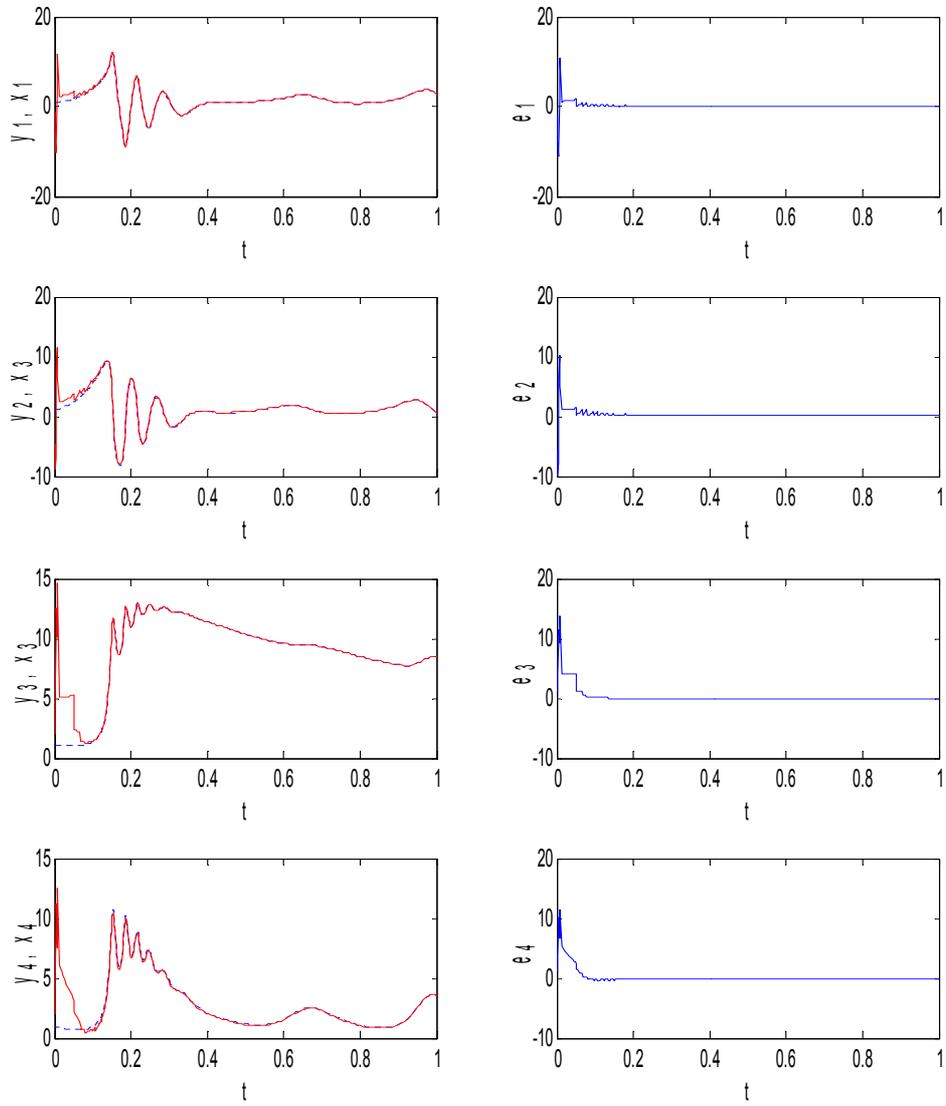
Figure 5: Synchronization of 4D chaotic system with impulsive control method for case I
