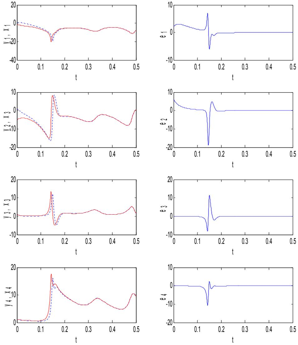
Figure 4: Synchronization of 4D chaotic system with passive control method for case II
