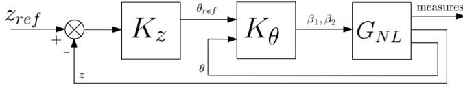
Fig. 2. Cascade control configuration for altitude control
