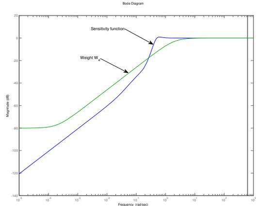
Fig. 4. Sensitivity functions of the pitch control
