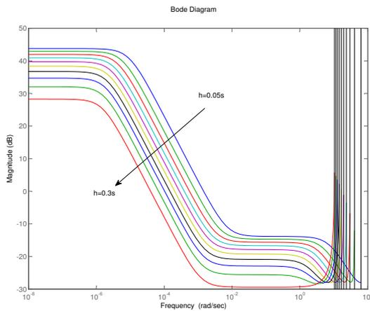
Fig. 8. Bode Diagram of the LPV polytopic controller
