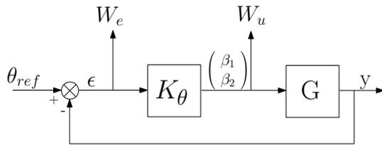
Fig. 3. Structure chosen for the control design
