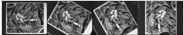
Figure 6: Example of images. A camera equipped on an arm robot was used to control the rotation angles precisely. Grayscale images were captured at 5 degrees increments through 90 degrees. The resolution of the captured images was 640 \times 480 .
