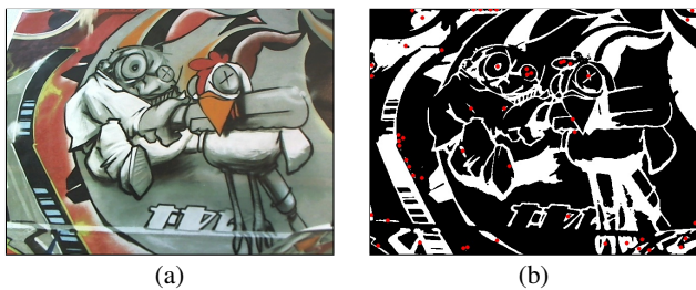
Figure 3: Applying word region detector [21] to Figure 1(a). Binarization by adaptive thresholding was applied to (a) an input image. (b) Few keypoints were extracted from segmented regions because most of the extracted regions were connected.
